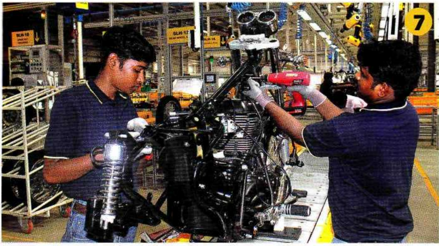
Wiring harnesses and chain are fitted with pre-torqued nut guns.
