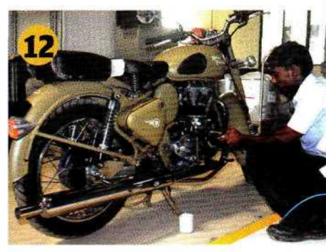
Final buffing done manually before the bikes are covered up and transported to dealers.
