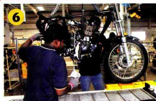
Bearings fitted into steering column with an air-gun before sub-assembled suspension column is attached.
