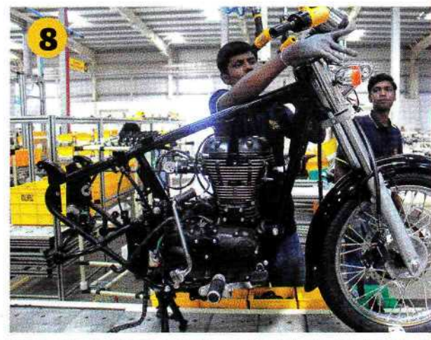
The famous circular speedometer cluster is then fixed before the handles and headlight casing are attached.
