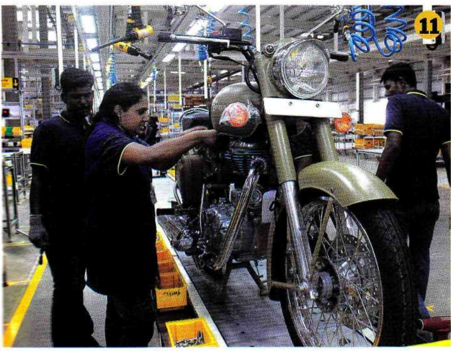
Wires are then connected and final checks are made before the vehicle is rolled out of the assembly line. Royal Enfield's ultimate goal is one motorcycle per minute in each shift.
