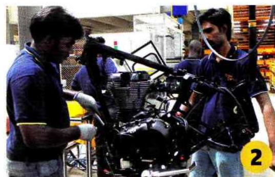
The engine and gearbox are bolted on to pre-fabricated frames. No fabrication takes place at the Oragadam plant.
