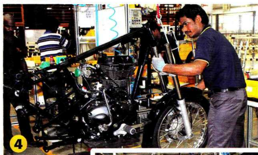
Bearings fitted into steering column with an air-gun before sub-assembled suspension column is attached.
