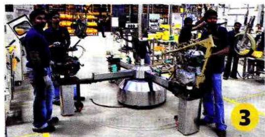
The engine and gearbox are hoisted on to the frame using this four-armed jig that helps save space at the start of the line.
