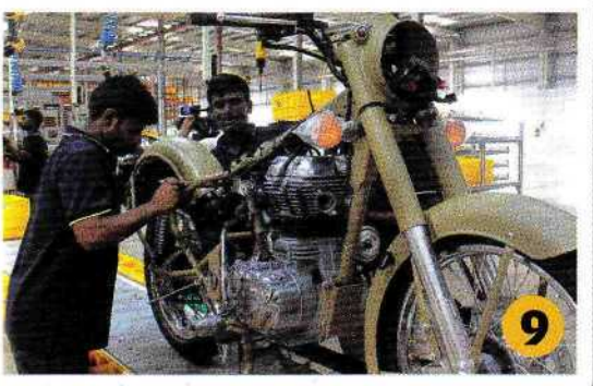
Rear fender attached to suspension with utmost precision; varies from twin-arm or twin gas-charged shock absorbers.
